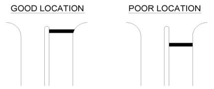
A stop line location close to the end of a median nose is a more natural stopping position than one some distance from the median nose. Not locating stop lines in their natural position will result in some drivers pulling past the stop line.
