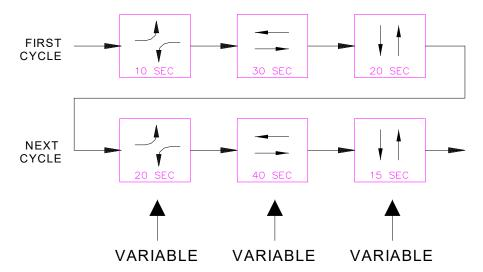
During a given time of the day, such as the AM rush hour, the green time provided to each phase can increase or decrease depending on the amount of vehicular demand. Vehicle demand at a fully-actuated signal is monitored by detection devices located on the various approaches to the intersection.
