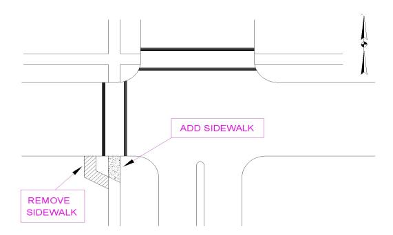
With the sidewalk and pedestrian crosswalk locations set, the next task is to locate the stop lines and associated lane lines and pavement arrows. Stop lines are white in color, typically 2 feet in width, and are usually located 4 feet behind any pedestrian crosswalk lines that exist:
