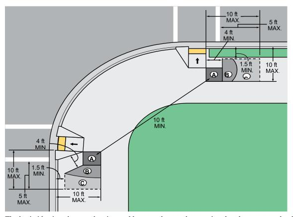
The basic idea is to keep pedestrian pushbuttons close to the crossing that they serve and at least 10 feet away from other pedestrian pushbuttons.
