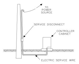
The electric service wire typically consists of 2 conductors, the black positive "power feed" wire and the white negative "neutral" wire. Sometimes a green ground wire is also provided.
