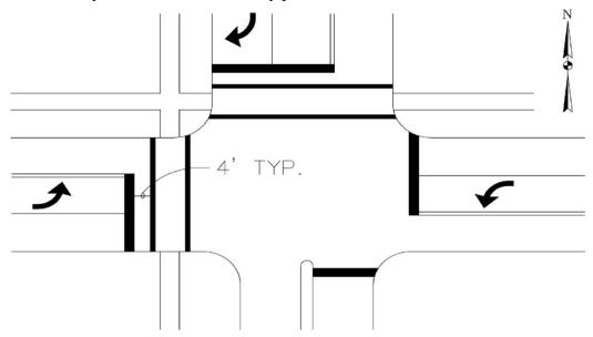
The "TYP." indication on a set of plans means "typical". In this case it means that all stop lines located behind crosswalks should be 4 feet away. It is always desirable to place the stop line behind the crosswalk; otherwise pedestrians will be required to cross between vehicles and crossing between vehicles is not considered a safe practice. When locating stop lines it is also desirable to place them as close as possible to the "natural" location at which drivers want to stop:
