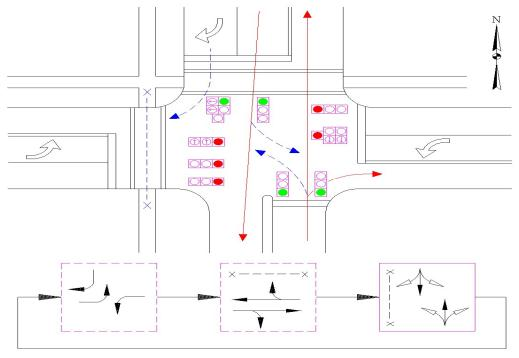
Note that all thru movements in this example are controlled by at least two signal indications:
