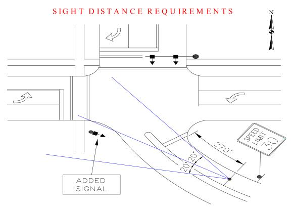
This drawing shows the use of a supplemental near side signal head to meet sight distance requirements. Supplemental near side signal heads are also useful when the "normal" heads are too far away from the stop line, or when a vertical sight restriction (such as an overpass) obscures the overhead signal indications.
