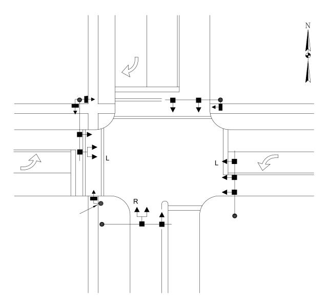
Note that, in this example, a separate pedestrian pedestal has been added to the southwest corner because the mast arm on this corner is too far away from the crosswalk to house the pedestrian head and pushbutton.
