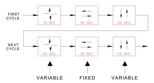
During a given time of the day, such as the AM rush hour, the green time provided to the side street phases and the main street left turn phases under semi-actuated control can increase or decrease depending on the amount of vehicular demand, but the green time provided to the main street through movements remains fixed. Vehicle demand at a semi-actuated signal is monitored by detection devices located in the main street left turn lanes and on the side street approaches to the intersection.
