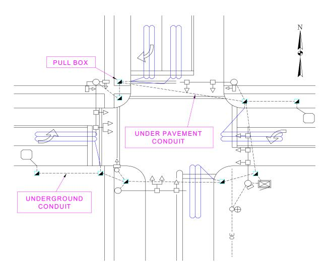
Many agencies like the idea of adding spare conduit runs during the initial installation of a signal in order to accommodate possible future expansion. Putting the spare conduit runs in "up front" is much less expensive, and less disruptive, then having to install additional conduits at a later date.
